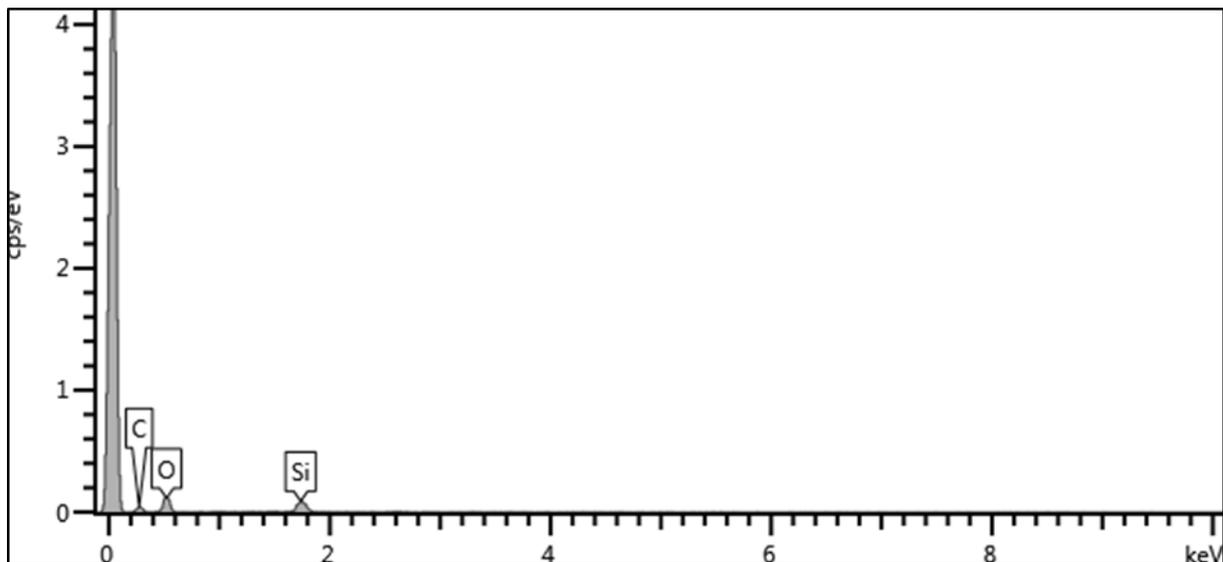
Figure 4. EDS spectrum of compressed OPT surface modified by silica nanoparticles and CTMS.
