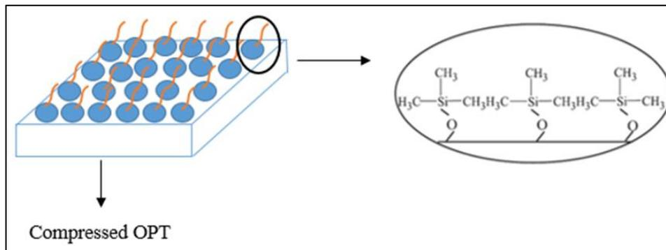
**Figure 2.** Schematic of compressed OPT surface after modified with CTMS.
