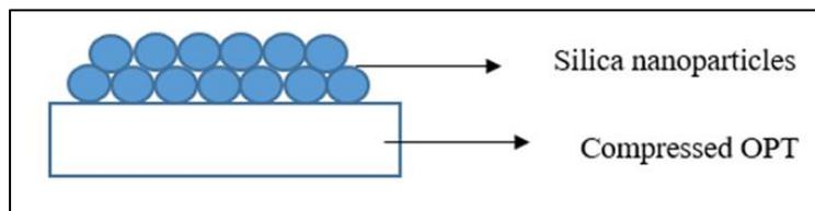
**Figure 1.** Schematic of silica nanoparticles deposited on compressed OPT surface.
