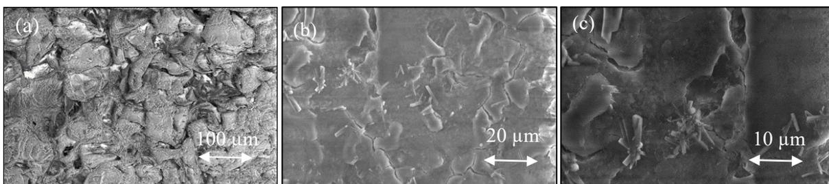
**Figure 3.** SEM images of OPT surface (a) before modification and the one modified with silica nanoparticles and CTMS at (b) low and (c) high magnification.
