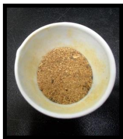
The SMS sample was placed in a crucible dish
