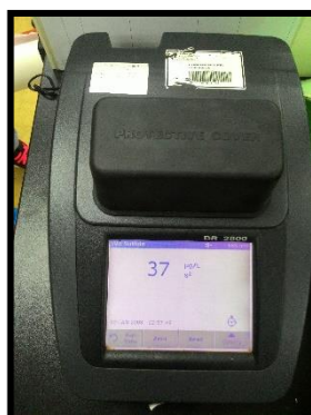
Then put the sample to read the sulphide content in it
