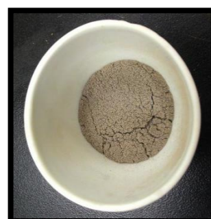
The chars obtained after carbonization
