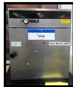
The SMS was placed in an Oven for 4h at 85 °C
