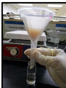
The sample was then filtered in a vial
