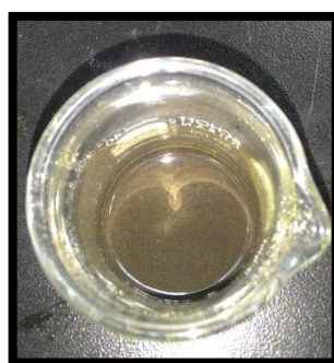
Impregnation the Chars with KOH solution
