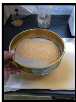
Then the SMS was sieved to 250 μm
