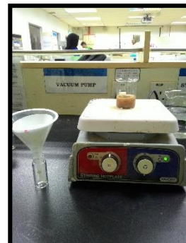
0.5g was mixed with sulphide solution for 3 min at constant stirring rate
