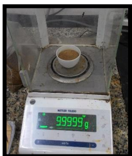
Weighing of the dried & sieved SMS
