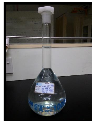
Dilute the \text{Na}_2\text{S} in 1L volumetric flask
