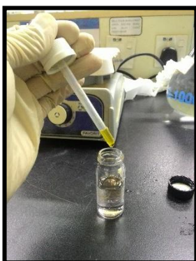
Reagent 1 & 2 was mix with the sample for sulphide testing
