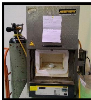
Carbonization of SMS at high temperature
