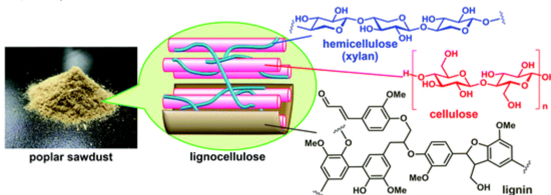
Figure 1: Scheme of the Lignocellulose Structure.
