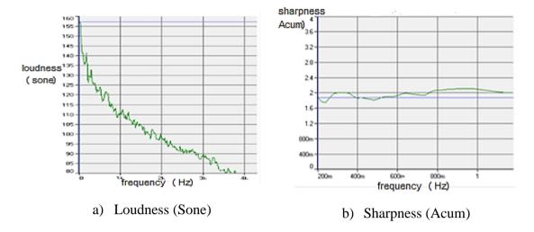
Figure 4. The sound quality metric loudness and sharpness (acum) of Axia on a pavement road surface at 2000 rpm.
