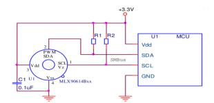
FIGURE 5: CIRCUIT DIAGRAM OF INFRARED THERMAL SENSOR (MIx90614)
