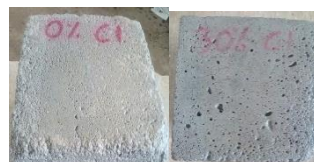
Figure 5. Physical Deterioration of Foamed Concrete at 1800hr
