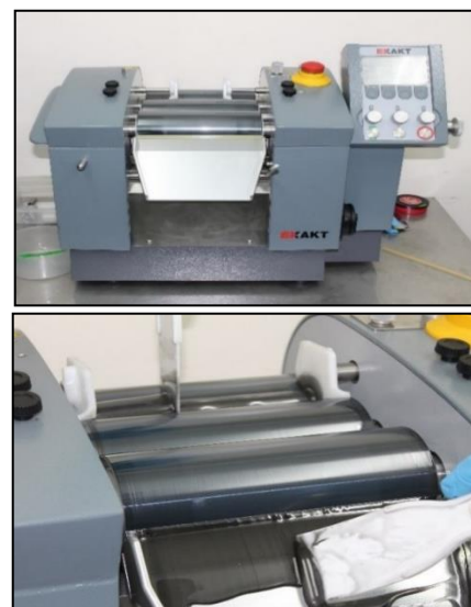
Fig. 1 Dispersion using three-roll mill machine.
