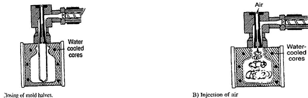
Figure 2.1 : Injection of air in blow mold
