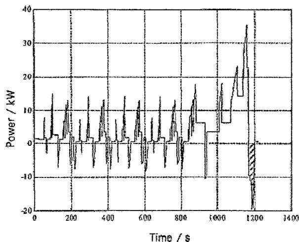
**Figure 2.4** Power profile of a 1130 kg car on NEDC
