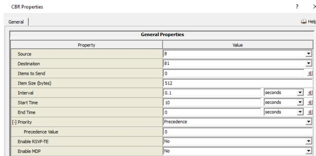
FIGURE 7. Configured parameters of the CBR data traffic generator.
