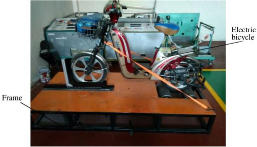
Fig. 3. The prototype of chassis dynamometer
