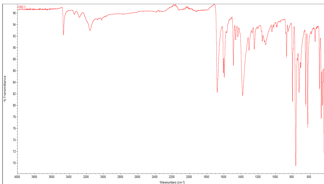
Figure 4. 8: FTIR for pure component CBZ
