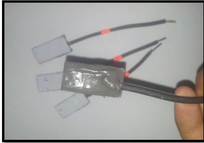
Figure 3.11: The uncoated surface of mild steel was been seal with epoxy hardeners
