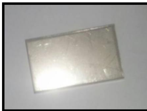
Figure 3.6: Mild steel after been polish with SiC paper (100, 200 and 800 grit silicon carbide paper)
