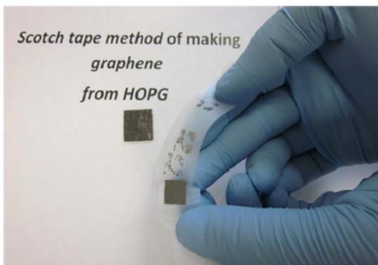
Figure 2.4: Micromechanical exfoliation of HOPG to produce graphene flakes:
