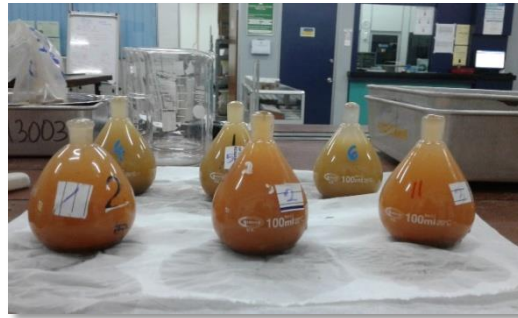
Figure 2. The density bottle, filled with distilled water and sample without stopper
