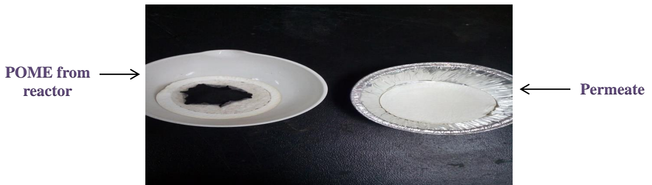
Figure 9: TSS test on 10th day
