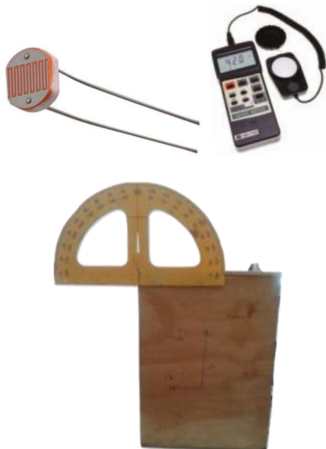
Figure 3.2: LDR, light meter and bench top enclosure
