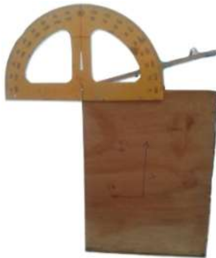
Figure 3.5: Opening angle of bench top enclosure
