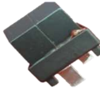
Figure 2.3: Example of Potting Unclean (Excess Resin)
