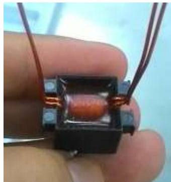
Figure 3.13: Second Potting and Final Hardening of Inductance
