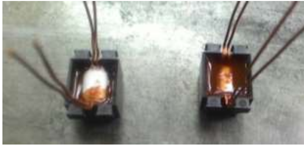
Figure 3.12: First potting of the inductance
