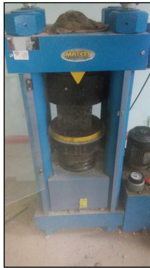
Figure 3.16 Compressive strength test
