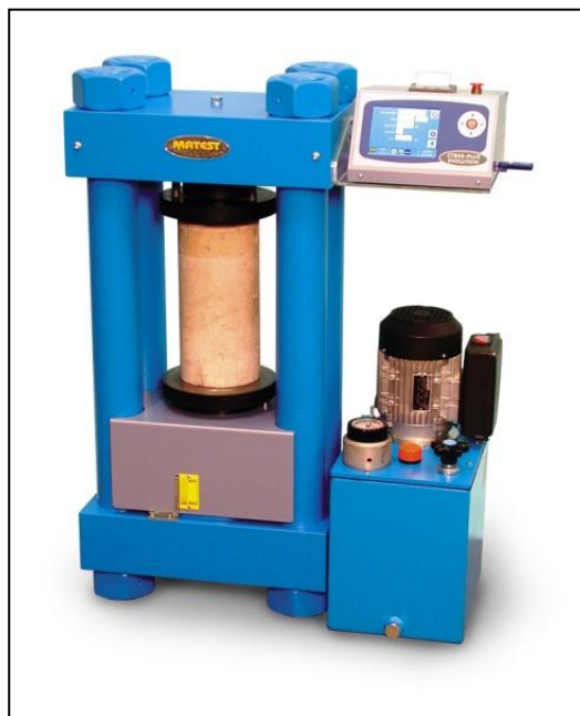
Figure 3.9 MATEST S.p.A. TREVILOLO 2408 COMPRESION MACHINE
