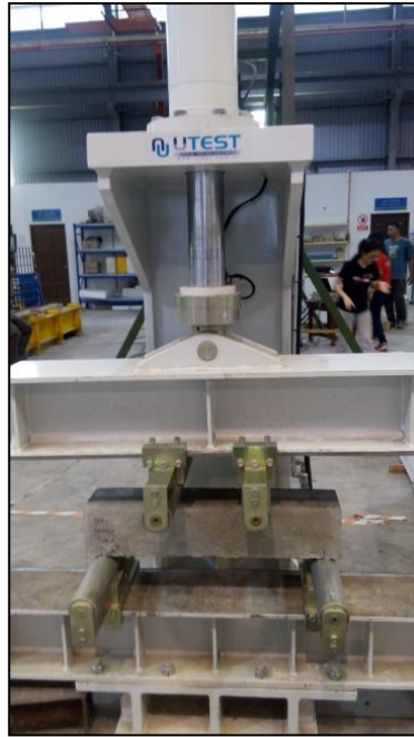
Figure 3.10 UTEST 300 kN AUTOMATIC FLEXURAL TESTING MACHINE
