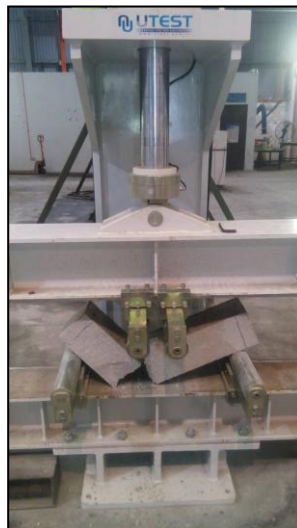
Figure 3.17 Flexural strength test
