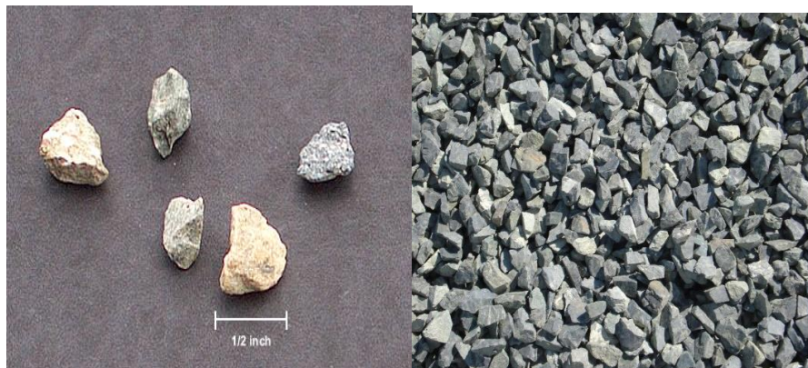
Figure 3.2 example of coarse aggregates
