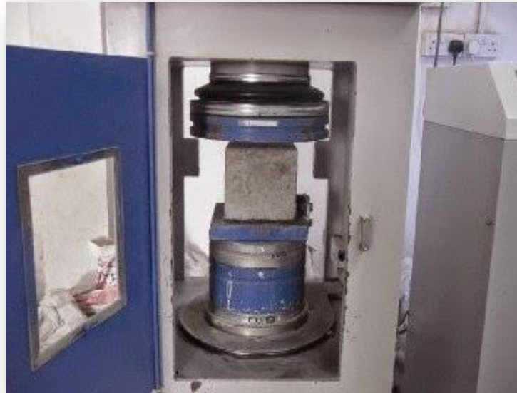
Figure 3.5 Compressive strength test equipment
