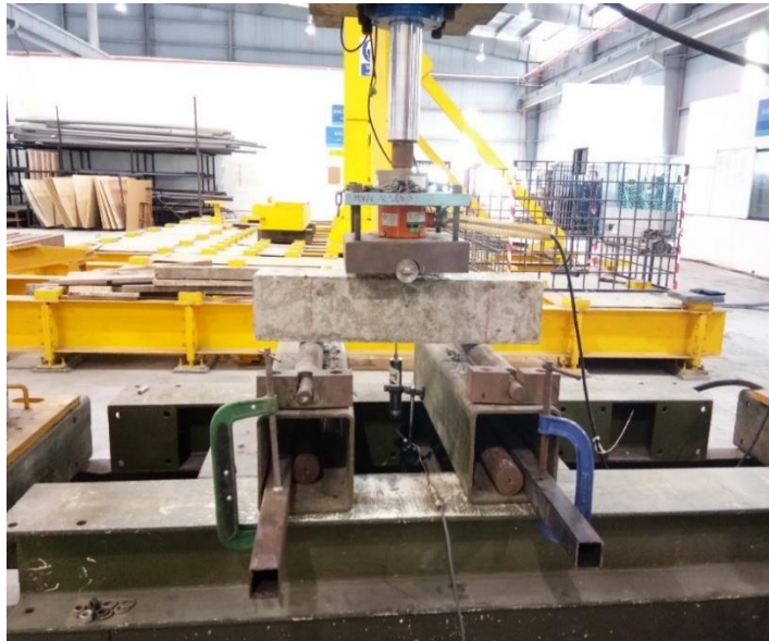
Figure 3.6 Flexural test equipment
