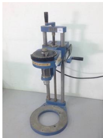
Figure 3.8 Vane shear test
