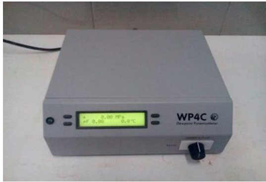
Figure 3.7 Chilled mirror dew-point technique
