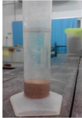
Figure 3.5 The apparatus set up for free swell test
