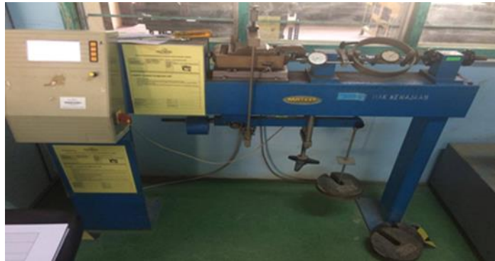
Figure 3.9 Direct shear test
