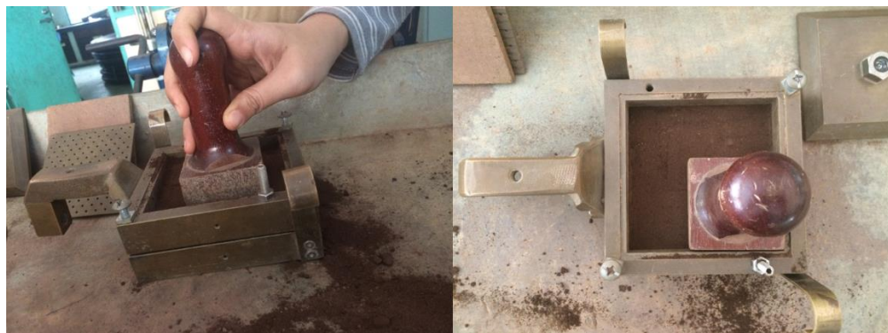
Figure 3.7 The soil sample was placed in cubic shear box
