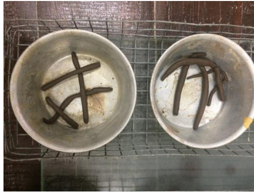
Figure 3.5 Apparatus set up for plastic limit test
