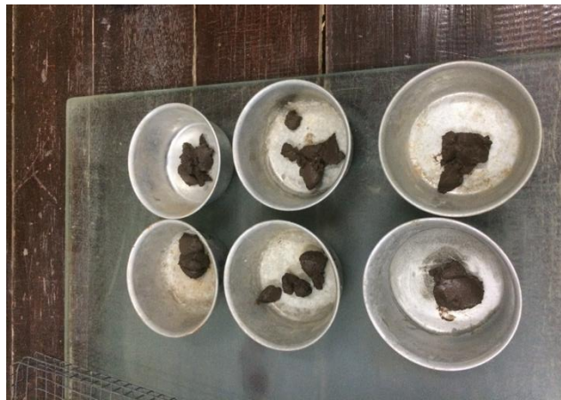
Figure 3.4 The apparatus set-up for liquid limit test
