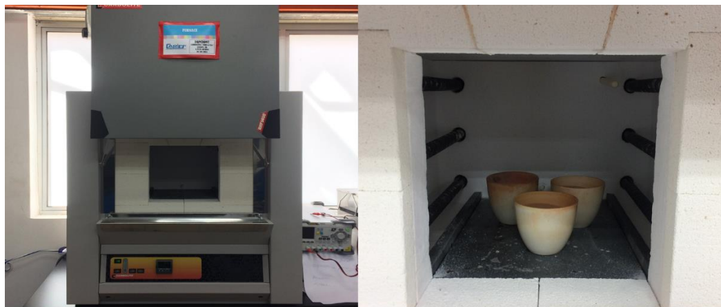
Figure 3.3 Preparation for burned soil sample using furnace
