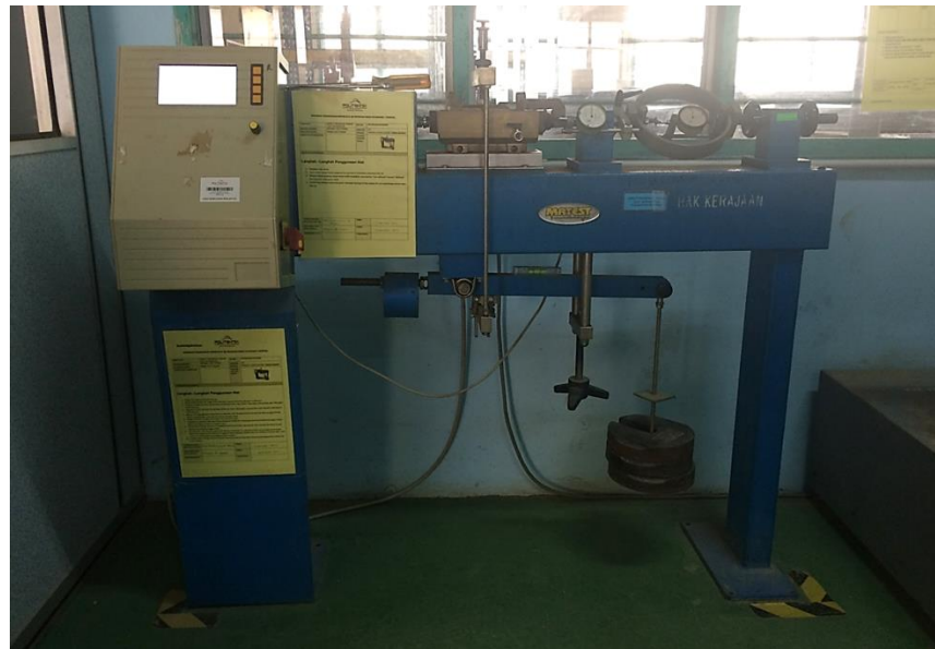
Figure 3.8 Apparatus set-up for direct shear test
