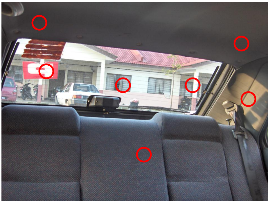
Figure 3.10 Temperature measurement spots at the rear panel and window
