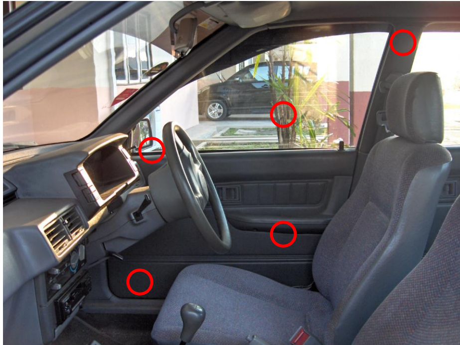
Figure 3.11 Temperature measurement spots at the front side panel and window
