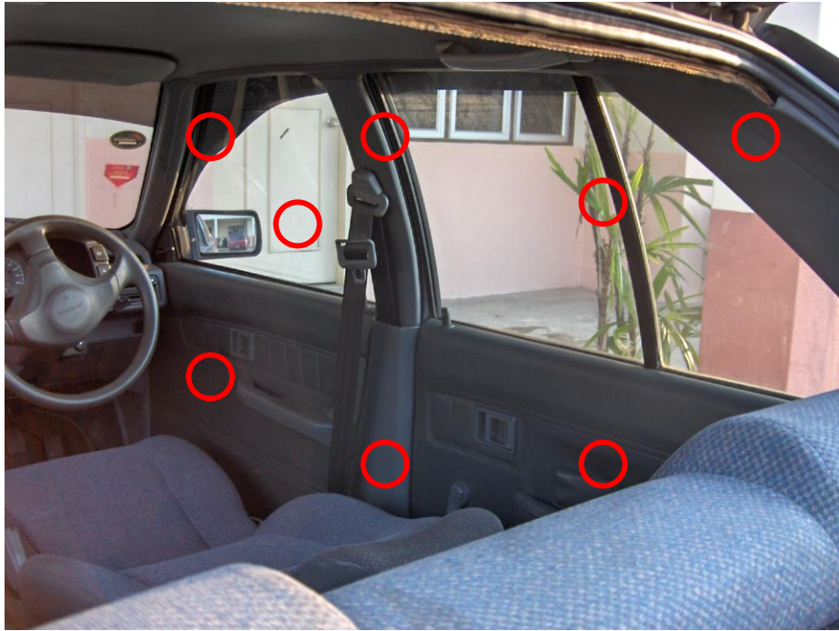
Figure 3.9 Temperature measurement spots at the front and rear side panels and windows
