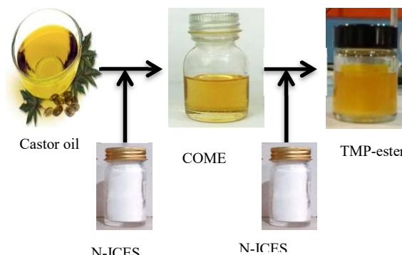
Fig. 4: Scheme of castor oil conversion to TMP-ester.
