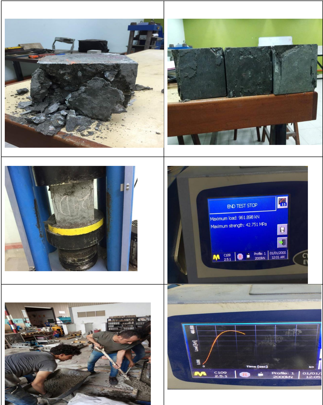
Figure B: cubes after testing with its result
