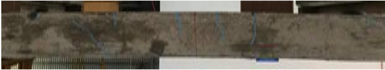
Figure 4.9: Failure mode and crack pattern of control beam
