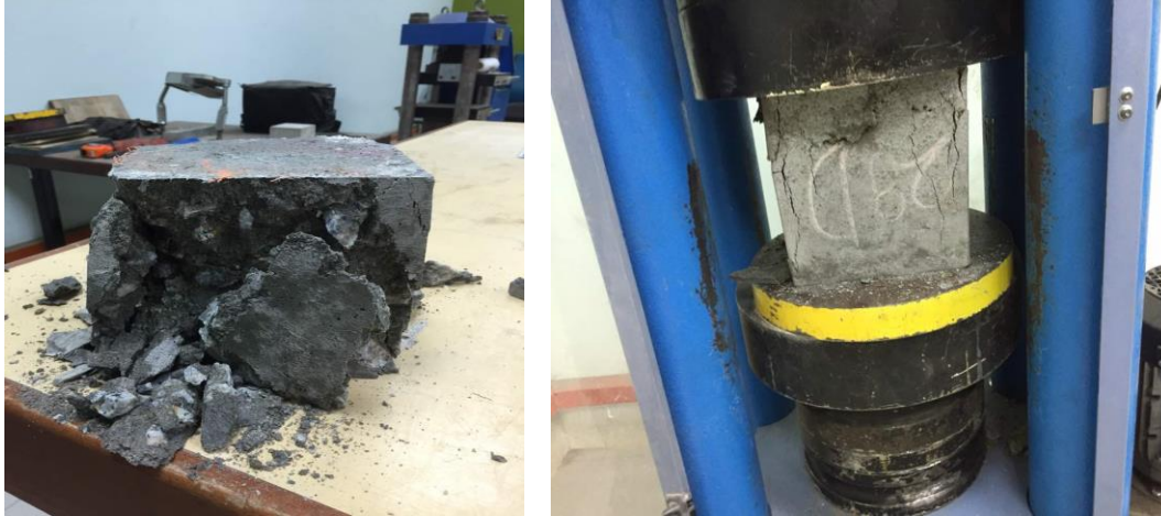
Figure 4.3: Cubes of Control Mix After Testing
