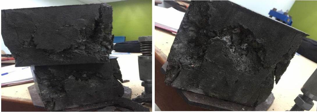
Figure 4.4: Cubes of RAC mix after testing
