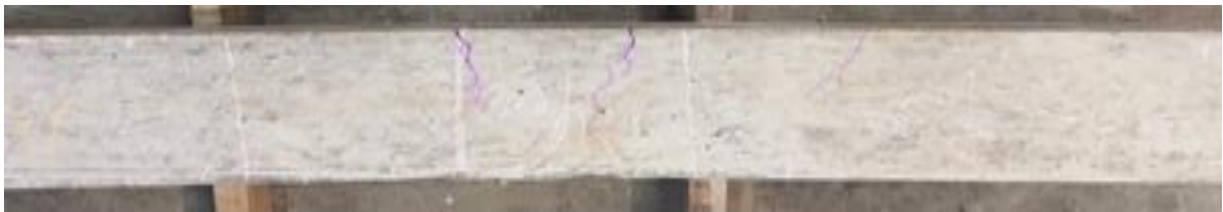
Figure 4.10: Failure mode and crack pattern of RAC beam
