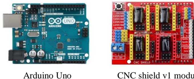
Figure 13: Basic pins and connection schematic of Arduino Uno and CNC shield v1 module [44]
