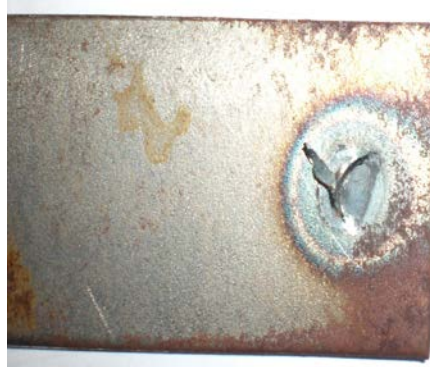
Figure 4.26: Crack during spot welding process
