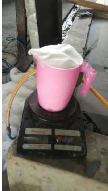
Figure 3.7 Measuring weight of 1 liter of foam
