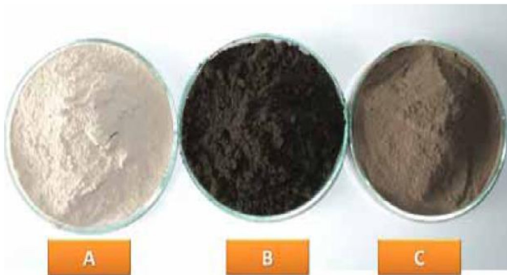
Figure 2.4.1 The features of fresh bleaching earth (A), Spent bleaching earth (B), and Reactivated bleaching earth (C)
