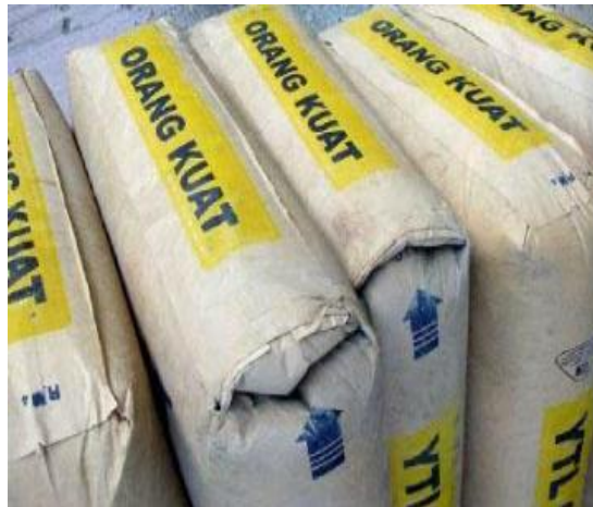
Figure 3.3.1 Ordinary Portland Cement
