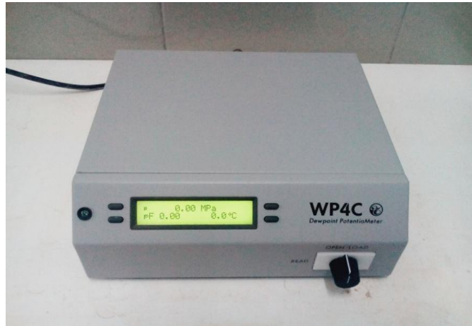
Figure 3.6 Apparatus set-up for Chilled Mirror Dew-Point Hygrometer Technique Test
