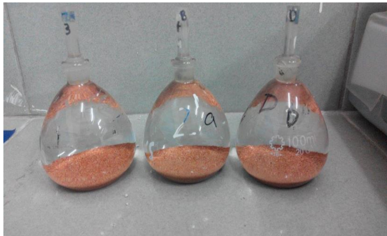
Figure 3.3 Apparatus setup for specific gravity test
