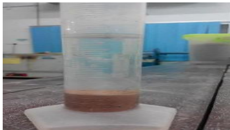
Figure 3.5 Free swell test apparatus setup
