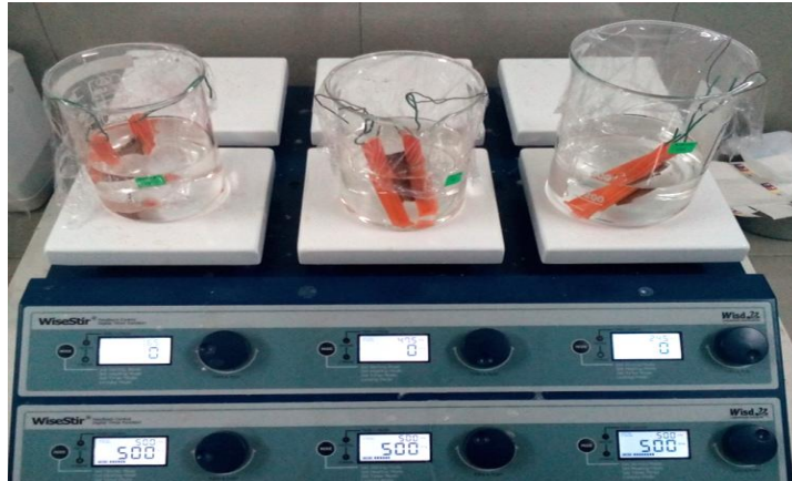
Figure 3.7 Apparatus set-up for Osmotic Technique Test
