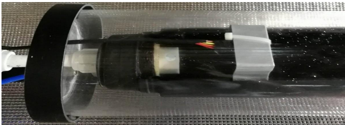
Figure 3.8: The sensor to estimate the seawater level in the absorber tube
