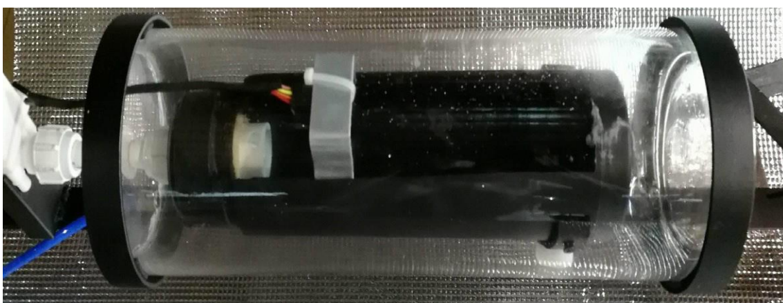
Figure 3.5: The absorber tube of the application of line focus concentrator for solar desalination process
