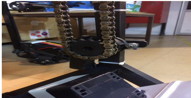
Figure 3.22: The motor chain of application of line focus concentrator for solar desalination process
