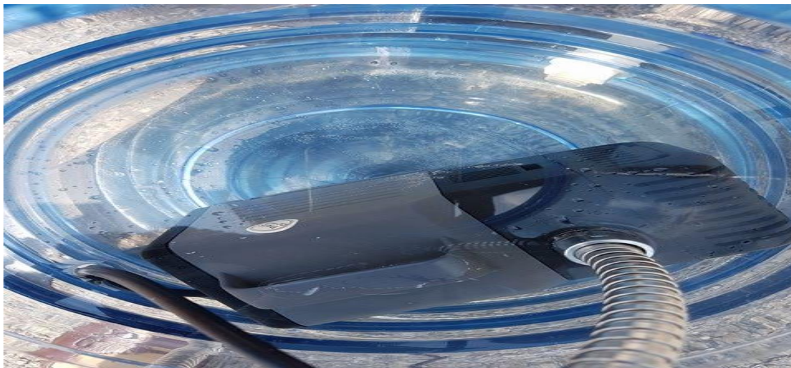
Figure 3.6: Water pump was immersed inside the seawater tank and connected to the inlet of the stainless steel
