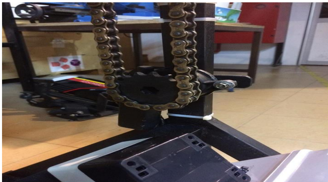
Figure 3.7: The motor chain of the application of line focus concentrator for solar desalination process
