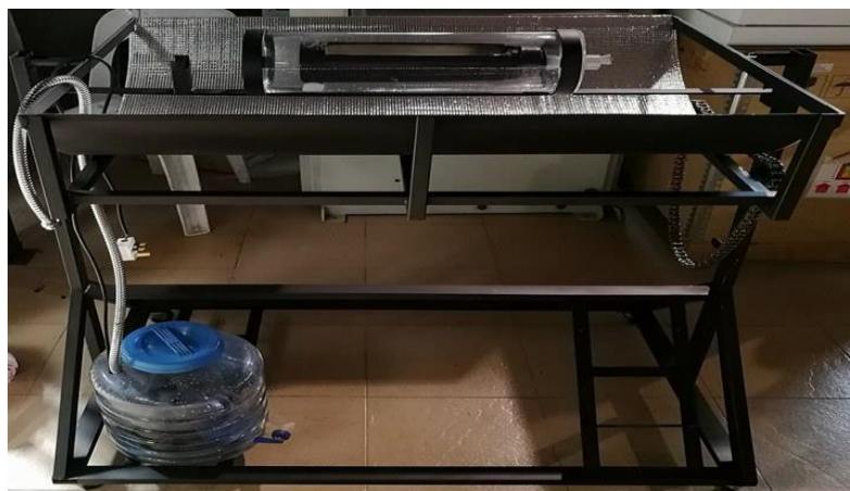
Figure 3.18: The support frame of application of line focus concentrator for solar desalination process.
