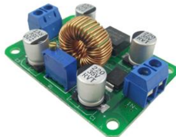
Figure 3.4 : Step Up Power Module
