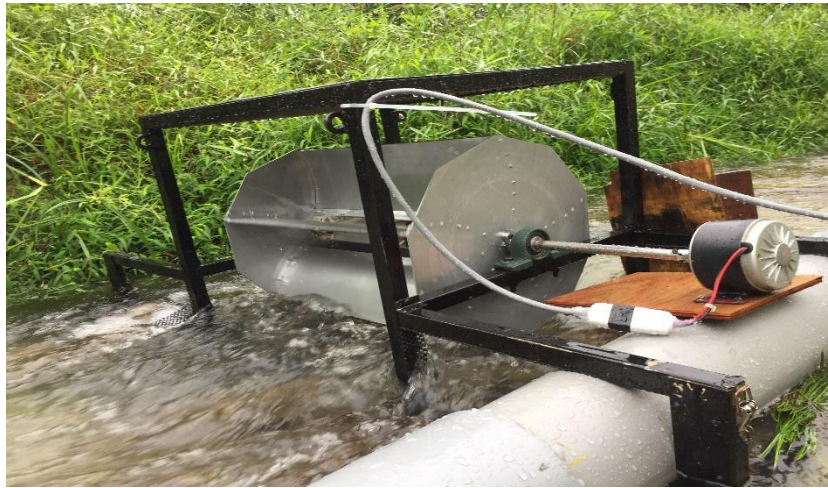
Figure 2.1 : The Hydrokinetic Turbines for Home Power
