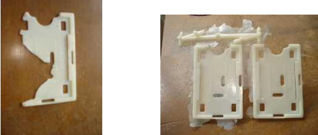
Figure 3.2: 2 types of major defects, right is flash defect and another is short shot.
