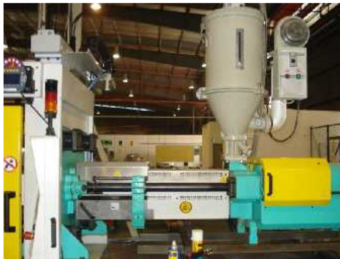
H. Injection Molding of each part.
