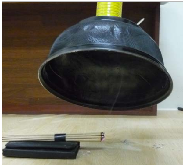
Figure 4.11: Fume Flow at 10cm Distance of Hood at 45° angle
