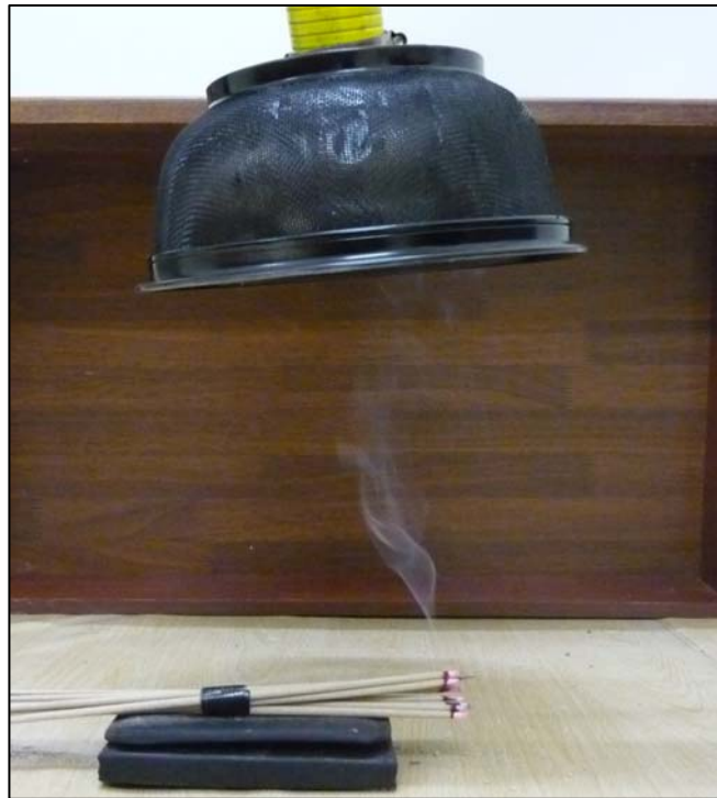
Figure 4.7: Fume Flow at 20cm Distance of Hood at 90° angle
