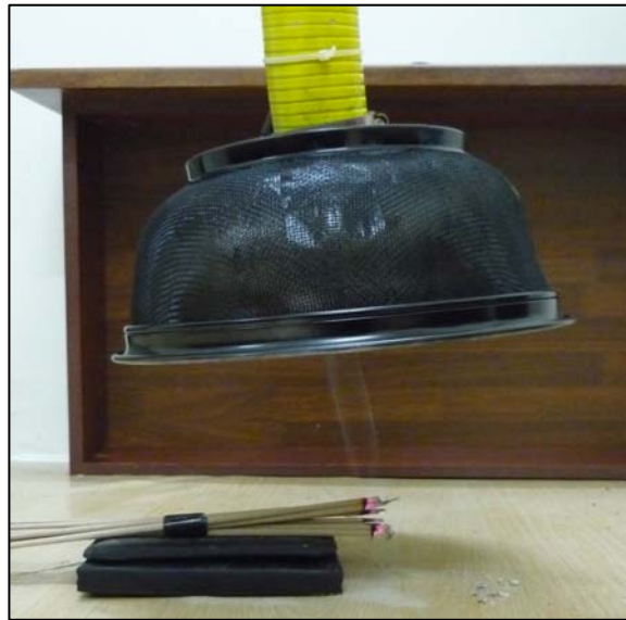
Figure 4.6: Fume Flow at 10cm Distance of Hood at 90° angle
