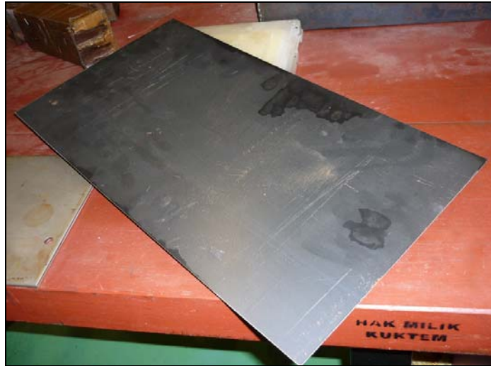
Figure 3.4: Sheet Metal Plate after Shearing Process
