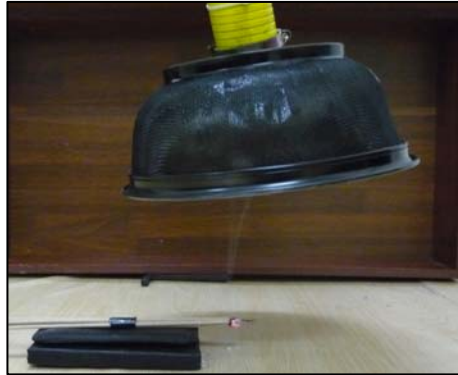
Figure 4.1: Fume Flow at 10cm Distance of Hood at 90° angle
