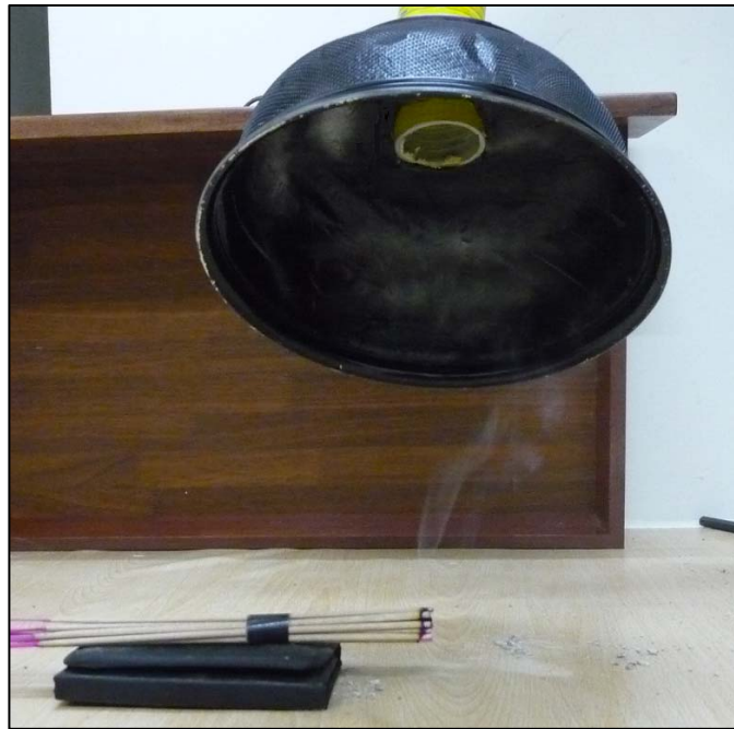
Figure 4.12: Fume Flow at 20cm Distance of Hood at 45° angle
