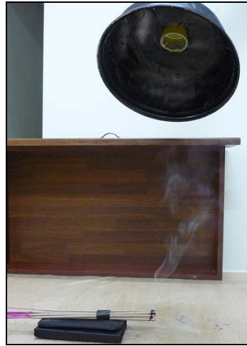
Figure 4.15: Fume Flow at 50cm Distance of Hood at 45° angle
