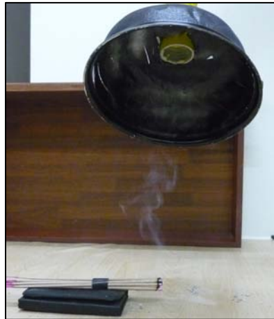
Figure 4.13: Fume Flow at 30cm Distance of Hood at 45° angle
