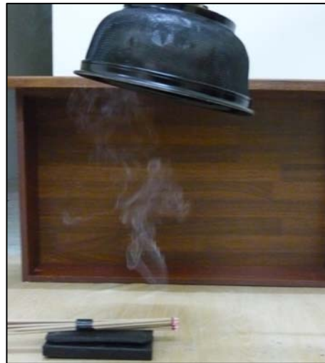
Figure 4.8: Fume Flow at 30cm Distance of Hood at 90° angle
