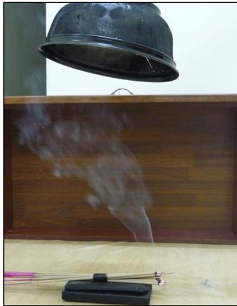
Figure 4.9: Fume Flow at 40cm Distance of Hood at 90° angle
