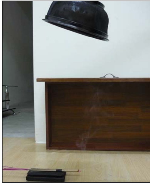
Figure 4.5: Fume Flow at 50cm Distance of Hood at 90° angle
