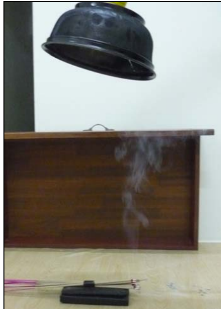
Figure 4.10: Fume Flow at 50cm Distance of Hood at 90° angle
