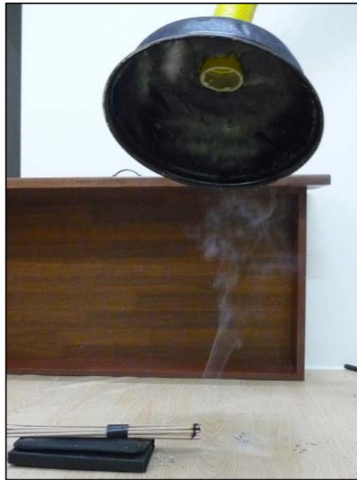
Figure 4.14: Fume Flow at 40cm Distance of Hood at 45° angle
