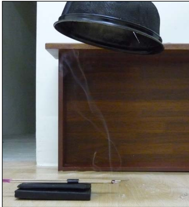
Figure 4.4: Fume Flow at 40cm Distance of Hood at 90° angle
