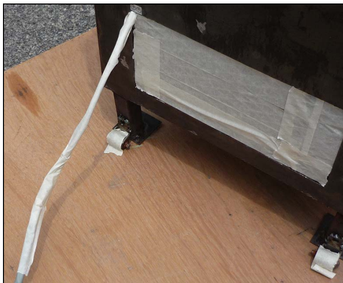
Figure3.8: Cover the Part which not been Paint
