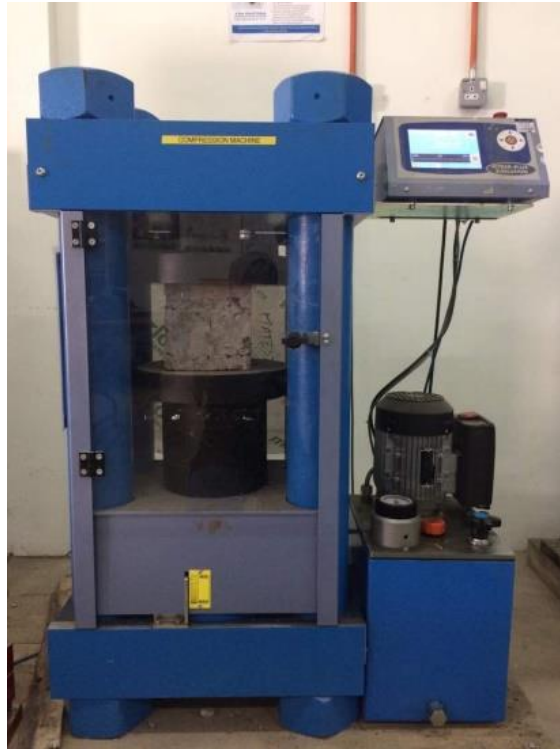
Figure 3.8: Compressive Strength Test Machine
