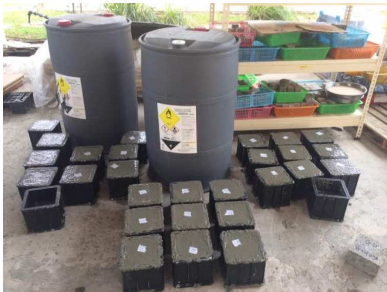
Figure 3.5: Concrete specimen after casting into the mould
