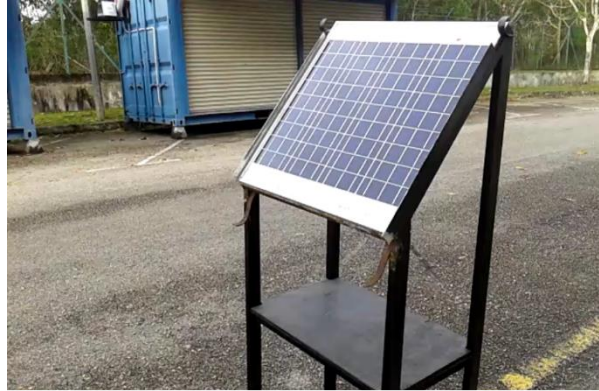
Figure 5.1 : The testing of PV solar panel output
