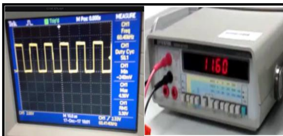
Figure 5.3 : The reading of output voltage by the buck-boost converter and the duty cycle for 12V
