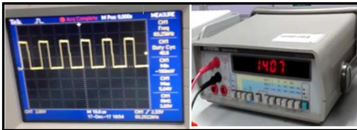
Figure 5.4 : The reading of output voltage by the buck-boost converter and the duty cycle for 17.2V
