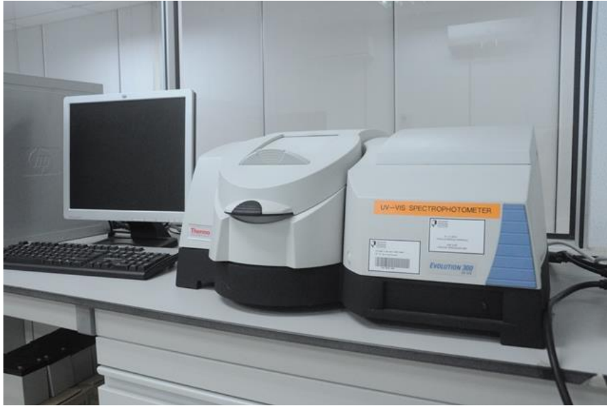
Figure 4.3: UV-visible absorption spectrometer used in UMP central lab.
