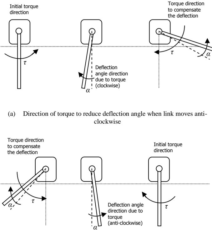
(a) Direction of torque to reduce deflection angle when link moves anti-clockwise
