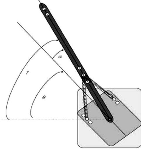
Fig.1. Description of the flexible joint manipulator system.
