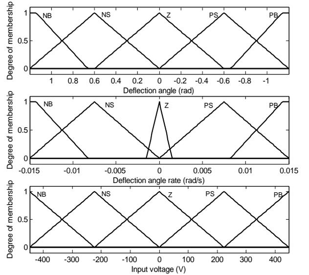
Fig. 4 Membership functions of inputs and output signals.
