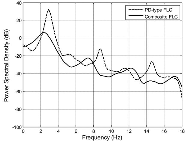
Fig. 8 PSD of deflection angle.
