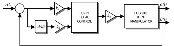
Fig. 2 PD-type fuzzy logic control structure.
