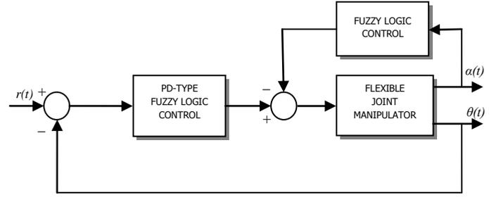
Fig. 3 Composite fuzzy logic control structure.
