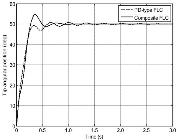
Fig. 6 Tip angular position response.
