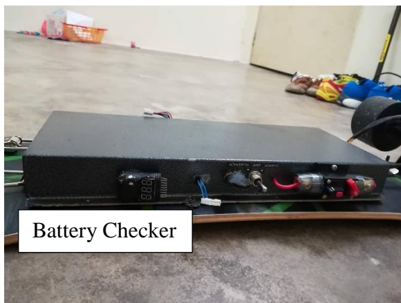
Figure 3.4.3. 7: Battery Checker Tester Low Voltage BB Buzzle Alarm
