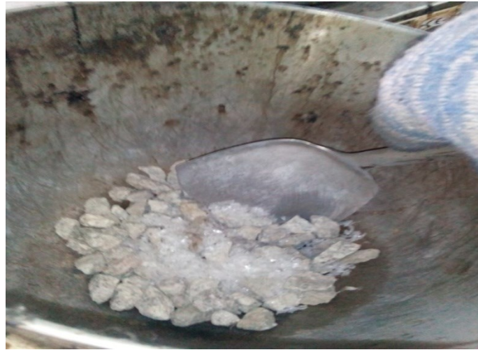
Figure 2. Process of aggregate coating
