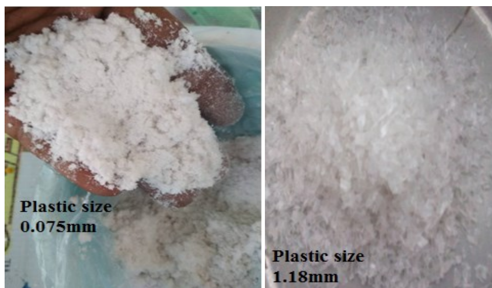
Figure 1. Plastic size 0.075mm to 1.18mm used to coat the aggregate
