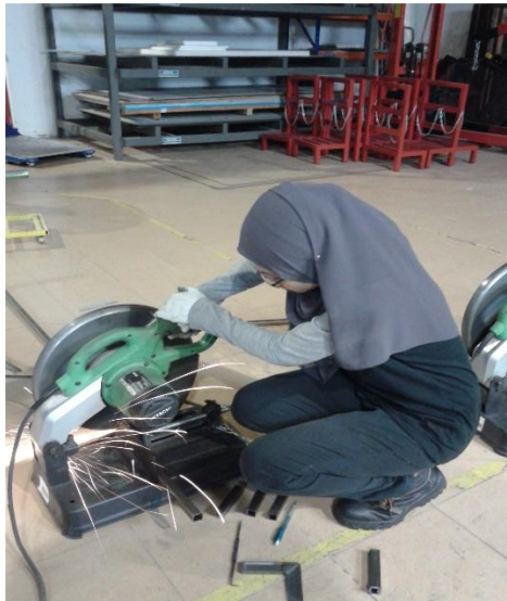
Fig.10 The hollow section steel was cut by using miter saw
