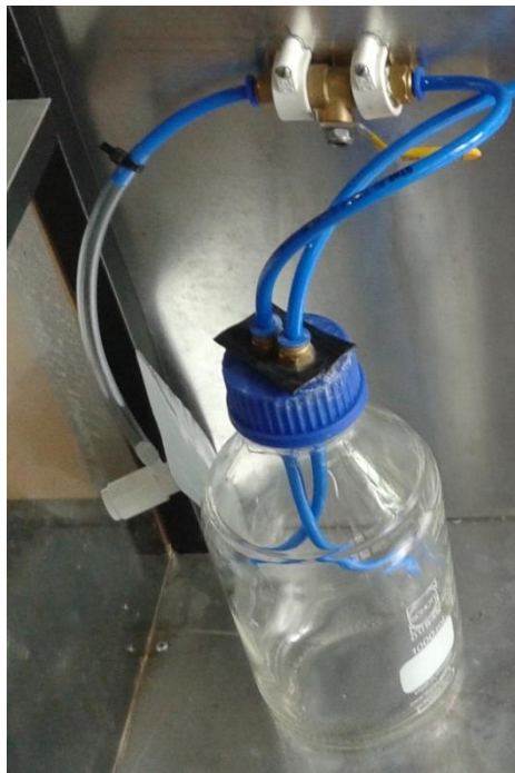
Fig.14 The bottle cap was attached with rubber to prevent air leakage
