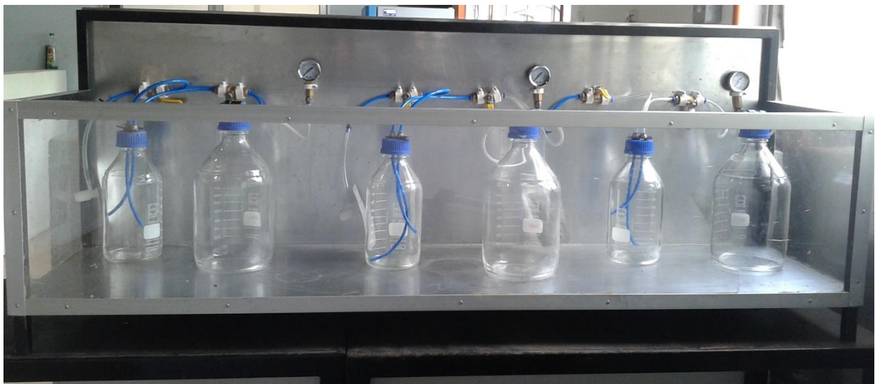
Fig.13 Dry fermentation reactor
