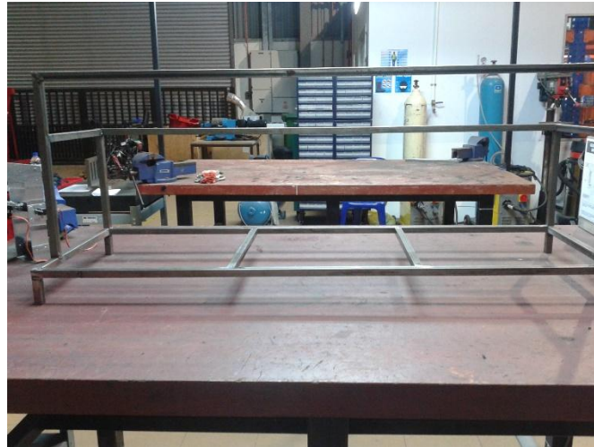
Fig.12 Welded frame for reactor container
