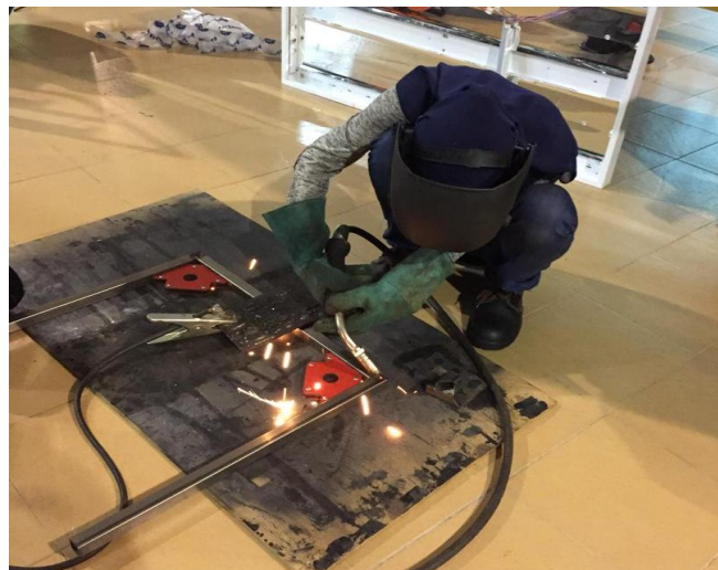
Fig.11 The hollow section steel was welded together to form a frame for making container
