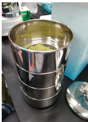
Figure 3.4: Sieves that been used to get consistent powder size of leaves powder
