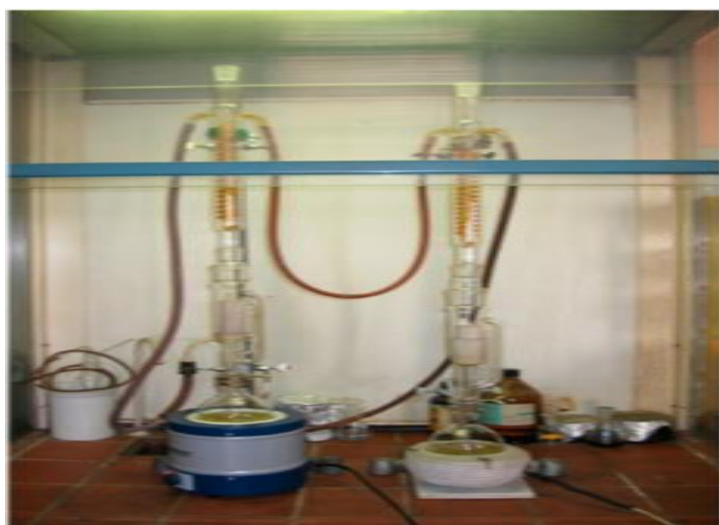
Figure 2.2 Soxhlet Extraction Method (Bankova, V. et al., 2016)
