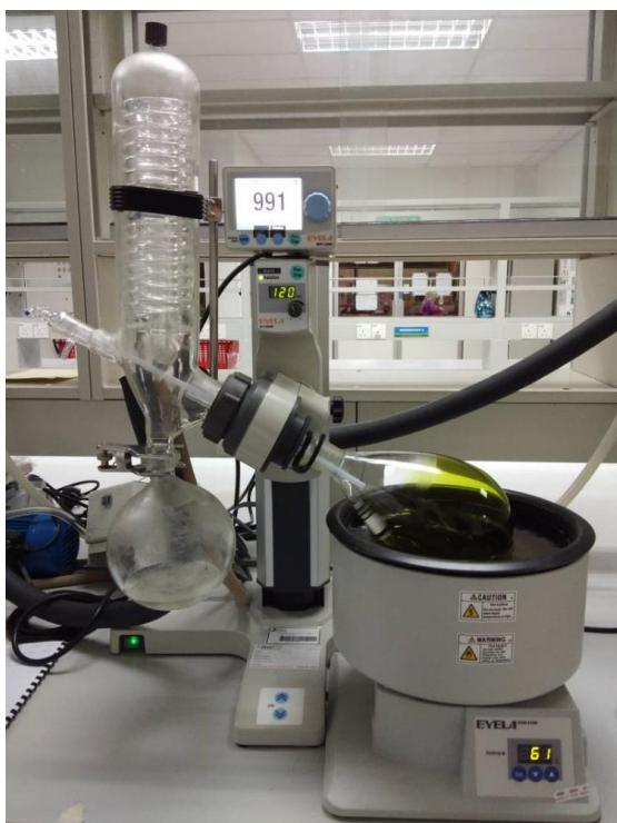
Figure 3.6 Ethanol was removed from stevia extract using rotary evaporator
