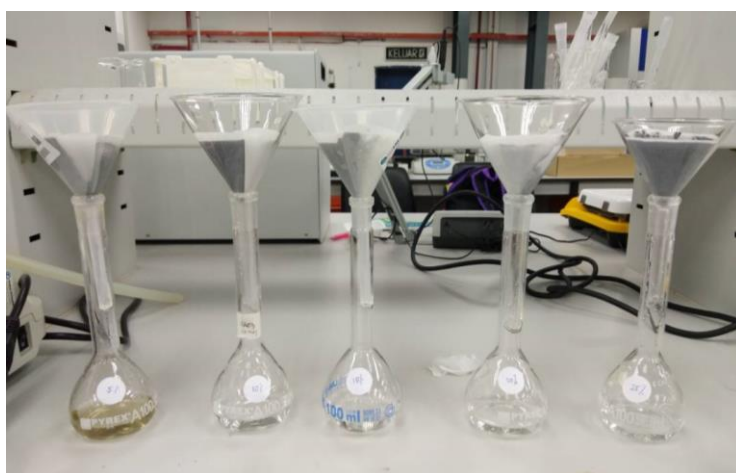
Figure 3.10 Mixture of stevia extract and activated charcoal were filtered through Whatmann filter paper.
