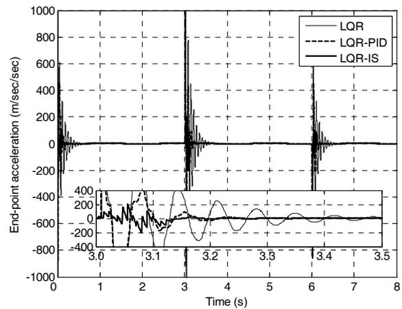
Figure 5. End-point acceleration response with LQR and LQR-PID and LQR-IS.
