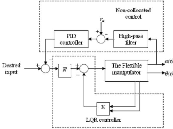
Figure 2. The LQR and non-collocated PID control structure.
