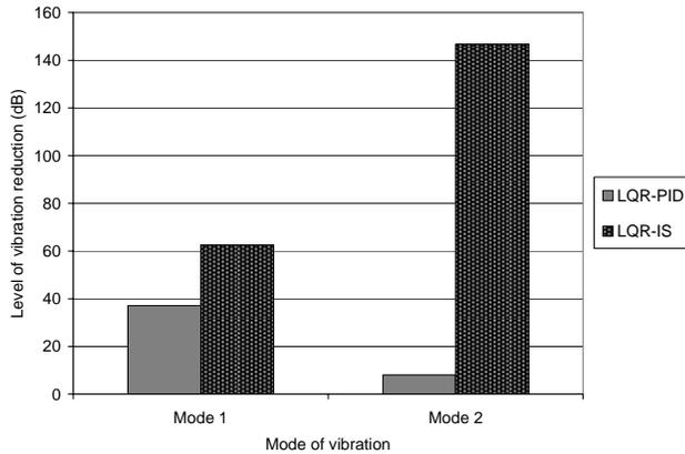
Figure 7. Level of vibration reduction with LQR-IS and LQR-PID. at the end-point of the manipulator.
