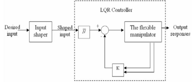
Figure 3. The LQR and input shaping control structure.
