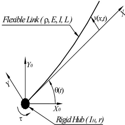
Figure 1. Description of the flexible manipulator system.
