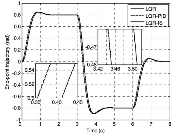
Figure 4. End-point trajectory response with LQR and LQR-PID and LQR-IS.
