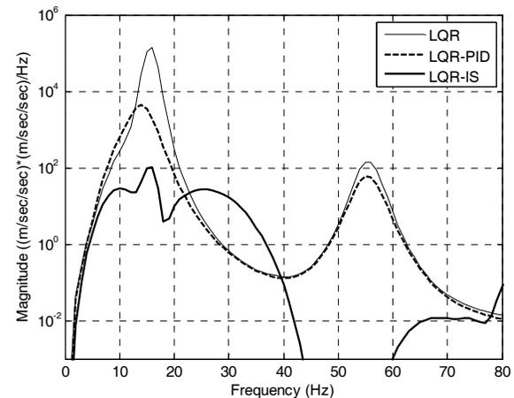
Figure 6. Power spectral density response with LQR and LQR-PID and LQR-IS.
