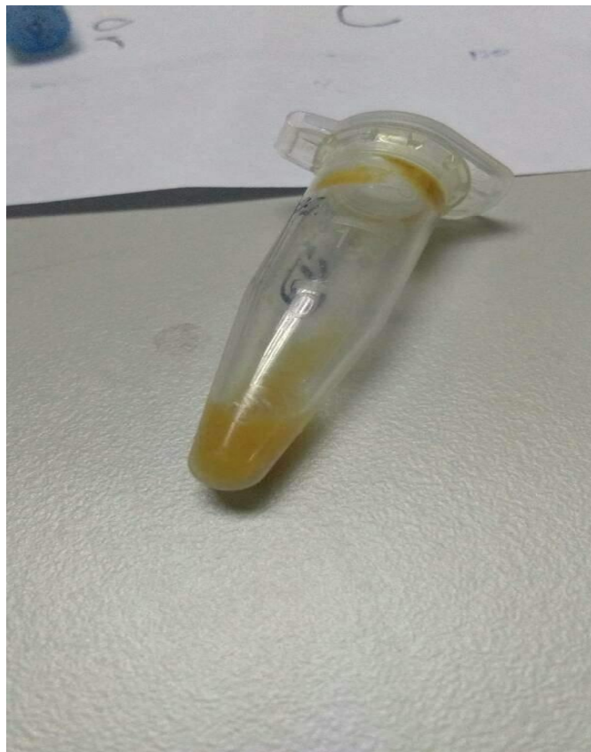
The picture shows the extract obtained after EEP was evaporated for 5 hours to remove ethanol residue.
