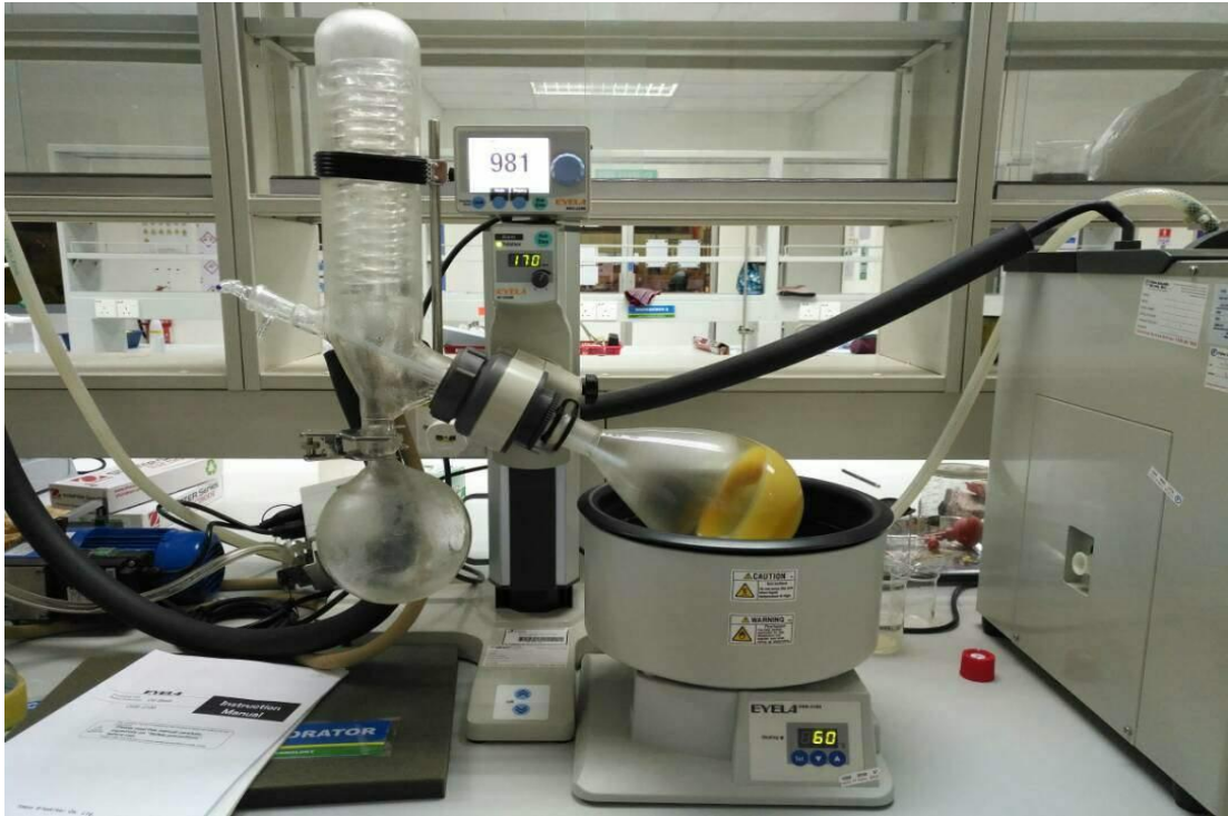
The picture shows rotary evaporator which is used to remove ethanol residue in EEP.
