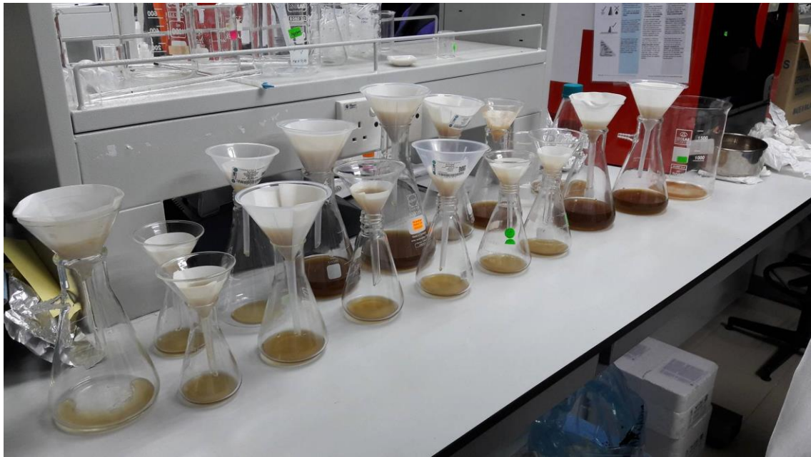
The picture shows process of filtration for WEP and EEP using Whatman size 1 filter paper.
