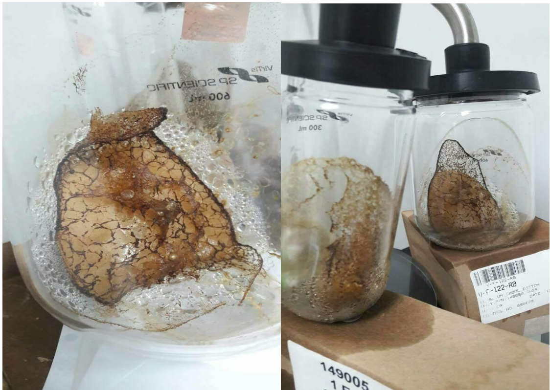
The pictures show the WEP were freeze dried to be changed in to powder. The pictures are the final product of 2 days of freeze drying.
