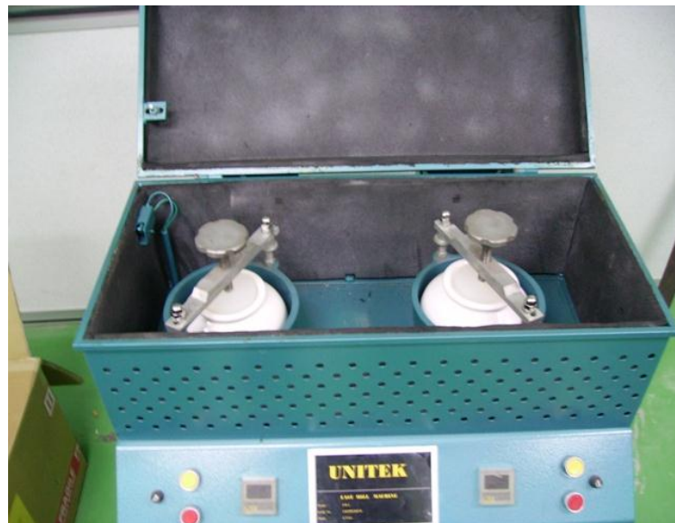
Figure 3.1: Milling process using ball milled
