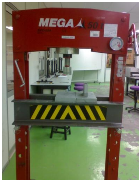
Figure 3.3: Compaction process using mold and die
