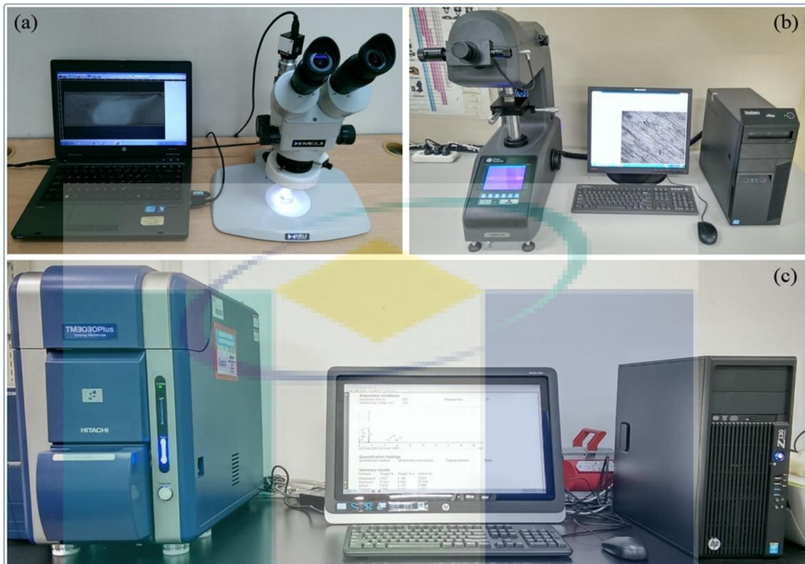
Figure 3.14 (a) The LED light-microscope, (b) The micro-hardness tester and (c) The SEM/EDS tabletop microscope
