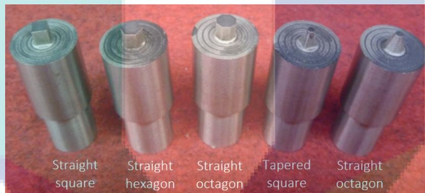
Figure 2.8 Straight and tapered probes
