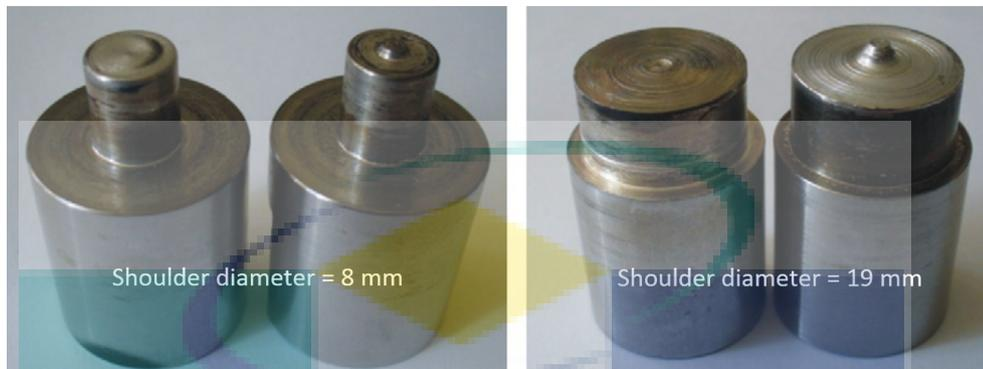
Figure 2.16 The pin and pinless tools with different shoulder diameters
