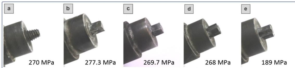
Figure 2.14 The five pin tool designs. (a) threaded tapered, (b) triangular, (c) square, (d) four-flute square, and (e) four-flute cylindrical
