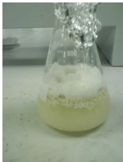
Precipitates formed once Ammonium sulfate added to the solution
