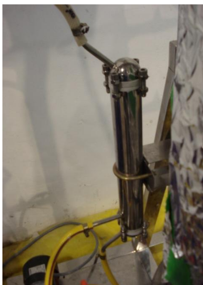
Figure 3.15: Cross flow Ultrafiltration Membrane (CUF) Unit
